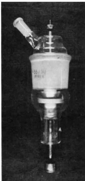
Fig. 1. Cell for measuring the dielectric strength of liquids.
